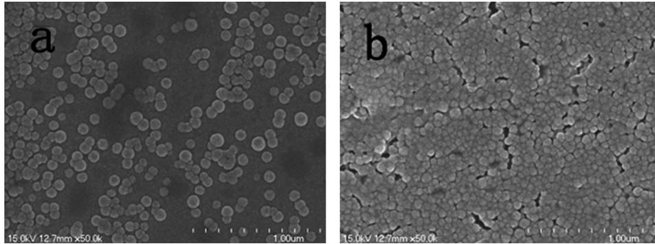
FIG. 1. The SEM image of (a) monodispersed PSNS and (b) PSNS array on PDMS.
