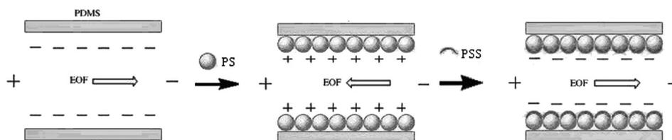
SCHEME 1. Schematic representation of the channel wall coating. The length of the channel is 3.50 cm.
