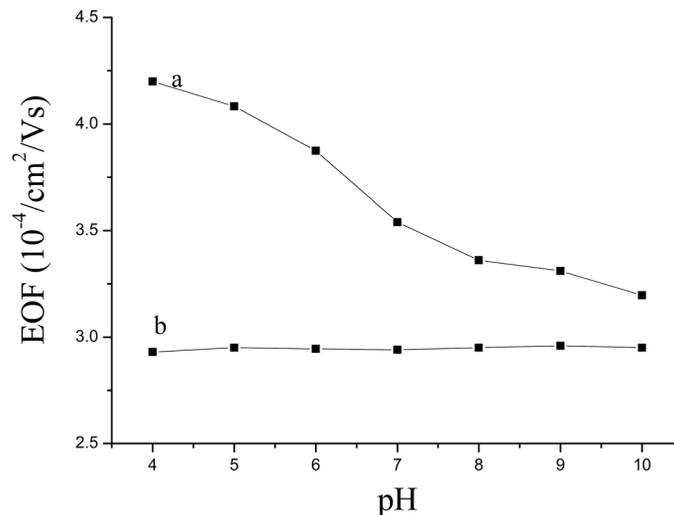
FIG. 2. The effect of buffer  $pH$  on EOF in (a) native PDMS microchannel and (b) PSNS/PSS coated PDMS microchannel under 1000 V of separation voltage with 20 mM PBS as running buffers.
