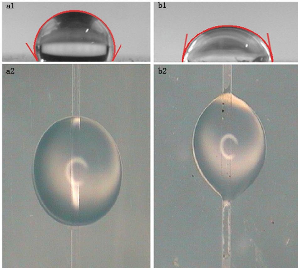
FIG. 3. The water contact angle on (a1) native PDMS and (b1) PSNS/PSS coated PDMS and corresponding droplet images (a2), (b2).
