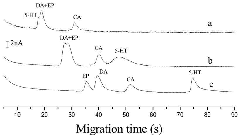
FIG. 4. Electropherograms of 50  $\mu\text{M}$  EP, DA, 5-HT, and 40  $\mu\text{M}$  CA on (a) native PDMS microchip, (b) PDDA/PSS coated PDMS microchip and (c) PSNS/PSS coated PDMS microchip. Sampled at 200 V for 1 s and detected at 0.60 V vs. Ag/AgCl.
